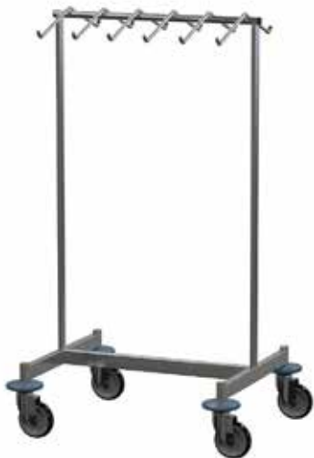
AX177 Lead Apron Rack 700 x 600 x 1420mm Stainless steel construction 12 apron hooks Corner buffers 125mmØ castors
